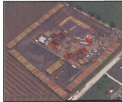
Conventional Drill & Frac Location
