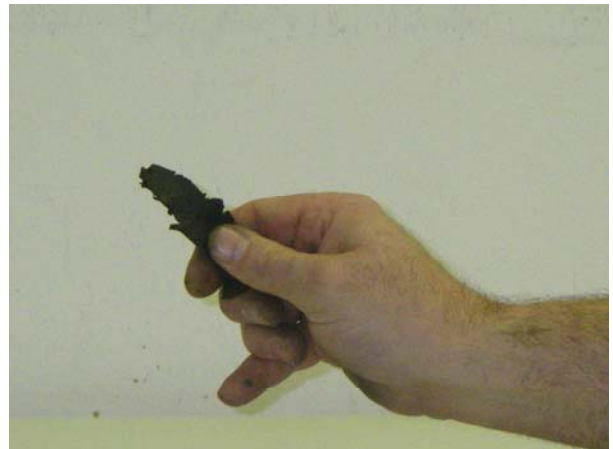
F – 2-inch ribbon formed due to higher clay content
