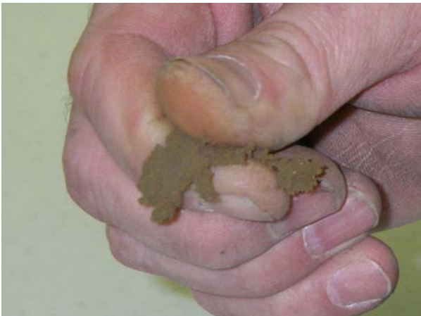
E – Less than 2-inch ribbon formed before breaking due to silt/loam content
