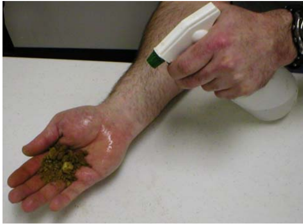
A – Sprinkle a few drops of water on the soil and knead the soil to break down its aggregates
