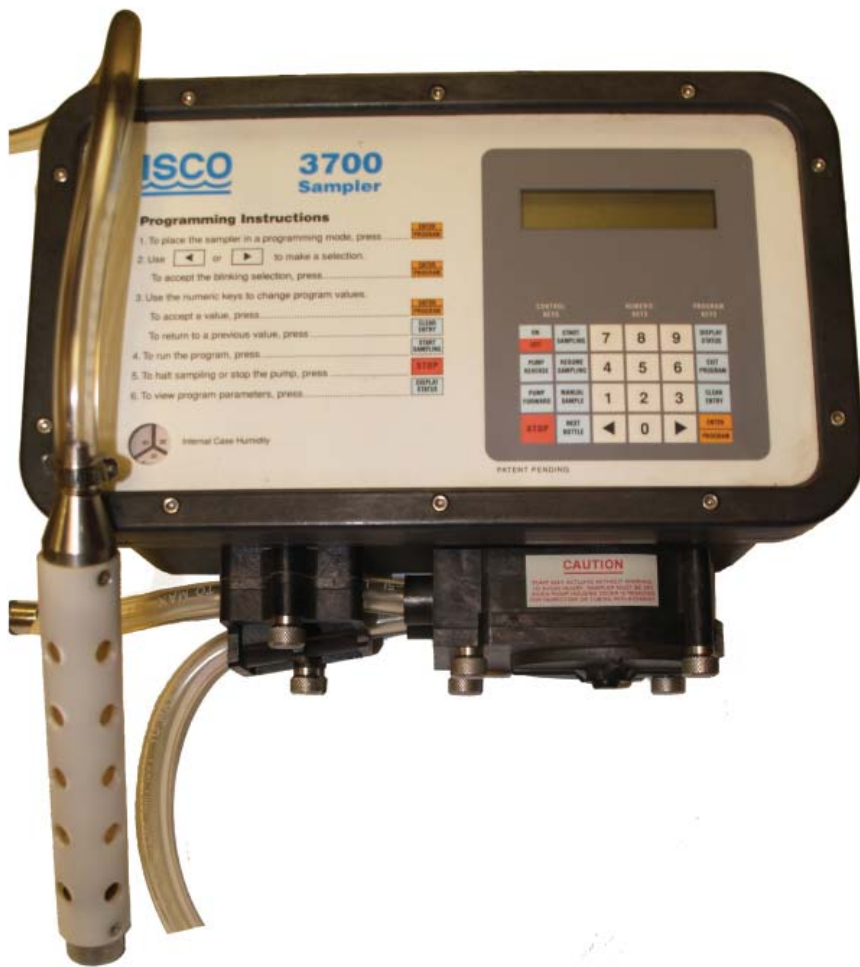
Figure 3.—An ISCO® 3700 sampler removed from its housing was used to obtain flowback fluid samples from the tank at 4-, 8-, 12-, and 16-foot depths. The strainer (i.e., intake) of the sampler is the perforated tube on the left front of the photograph. Photo by Frederica Wood, U.S. Forest Service.
