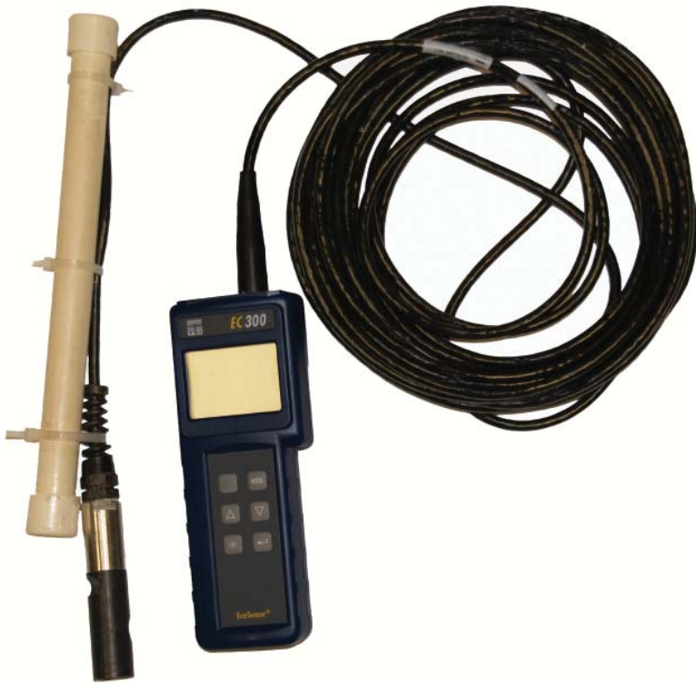
Figure 2.—The capped PVC pipe attached to the conductivity cell cable contains water that was used to provide extra weight to the cell to keep it from becoming buoyant when lowered into the flowback fluid in the tank. Photo by Frederica Wood, U.S. Forest Service.
