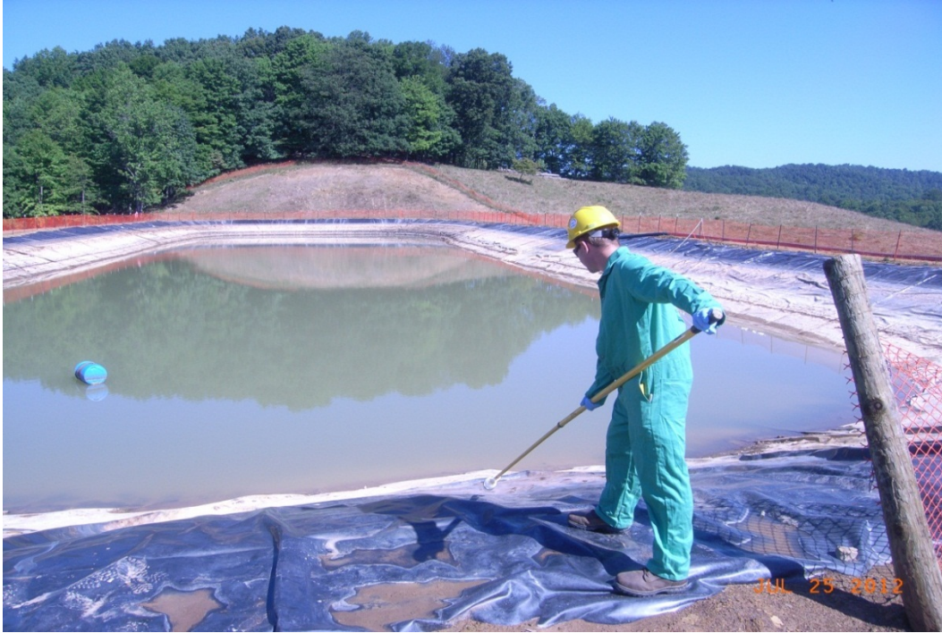
Figure 8: Donna Pad Pit Sampling of Hydraulic Fracturing (Makeup) Water
