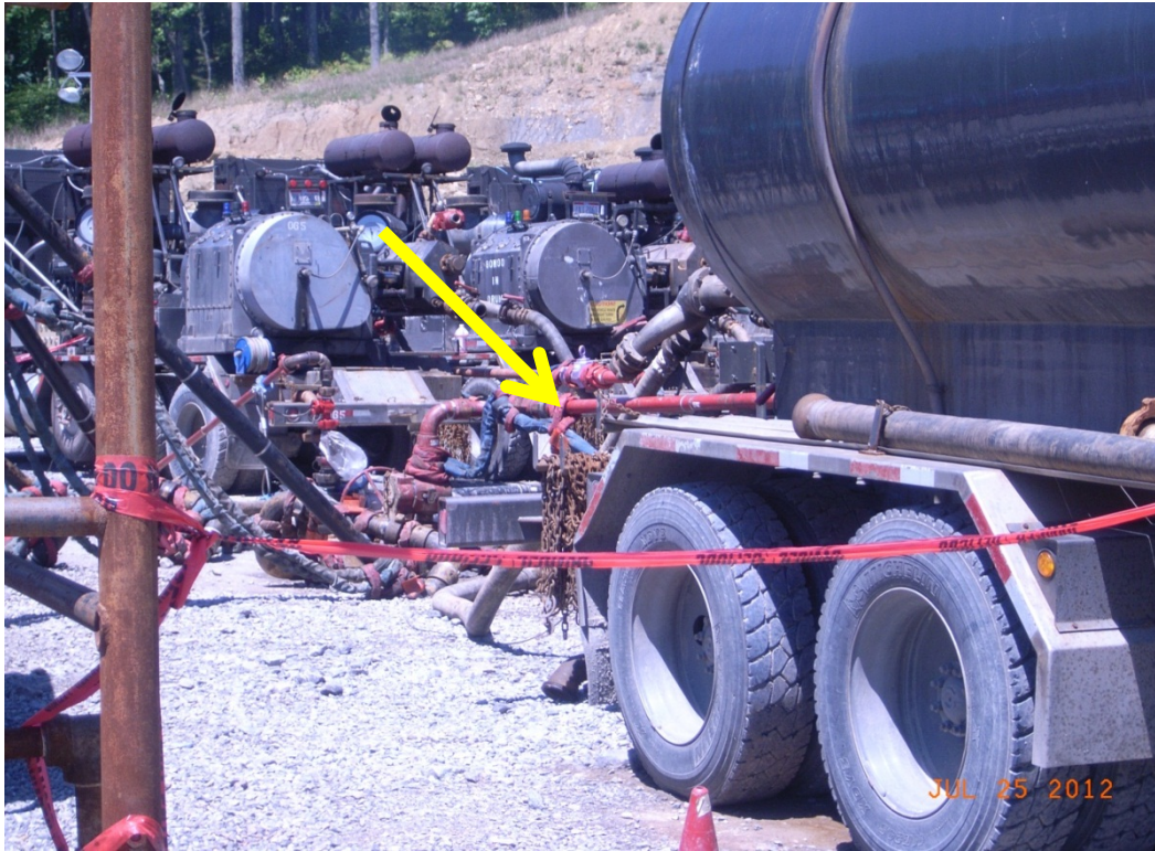
Figure 10: Sampling Location of Hydraulic Fracturing Fluids
