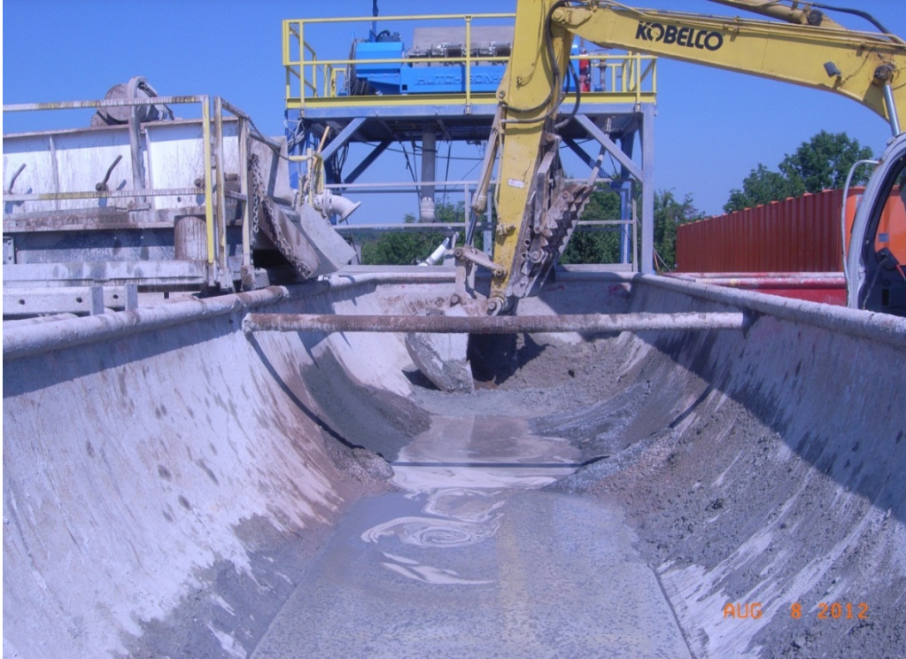
Figure 5: Lemons Pad – Shaker Table Solids
