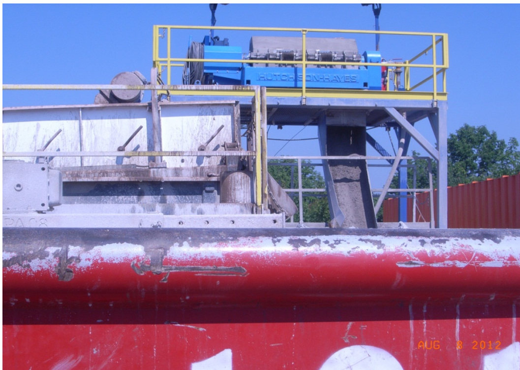
Figure 7: Mills Wetzel Pad #2 Shaker Table (where samples were pulled)
