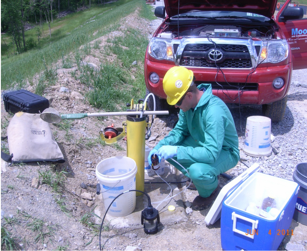
Figure 19: Collection of Groundwater Sample from Consol/Noble Centralized Pit SHL2
